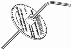
Thread hex wrench into minidial to gage adjustment as you turn.
